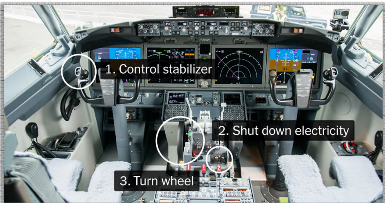
Figure 5. Boeing’s hazard assessment assumed that, in response to an MCAS malfunction, pilots would perform multiple tasks, like those above, never previously required in any other Boeing plane, in under three seconds.
