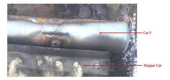
321. The Norfolk Southern team understood that the hopper car containing plastic pellets generated radiant heat that slowed Car 5's cooling. This is "firefighting 101" as one Norfolk Southern-friendly witness explained: that hopper "car up against" Car 5, "there's going to be some heat transfer" though he could not say the exact amount, "there will be some heat transfer, absolutely." The Norfolk
